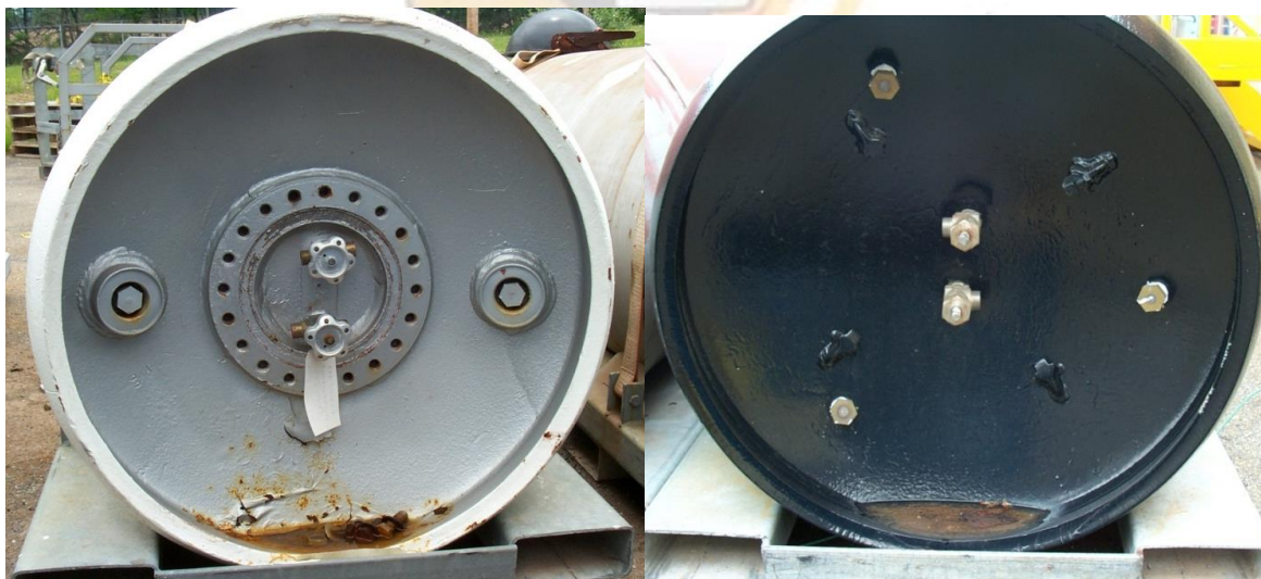
Highly toxic ton unit for Phosgene, Cyanogen Chloride on left. Has vapor tight dome cap and PRD seal cap.
