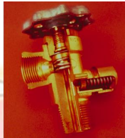
CG-7 Springloaded PRD, Used for LPG gases, butane, propane, isobutane
