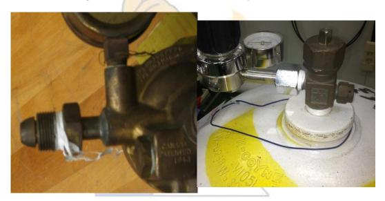
Use of teflon on the threads can cause the connection to leak as the cylinder pressure pushes against the valve outlet causing the fitting to move away from the nipple or gasket. At high pressures, the Teflon tape can also cold flow
