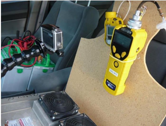
Gas Sensors in Car with Go Pro
