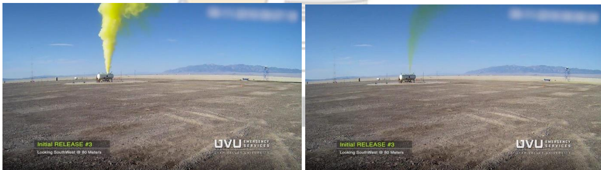
Figs. 14 & 15: Vapor Venting from 20 Ton Chlorine Tanker
