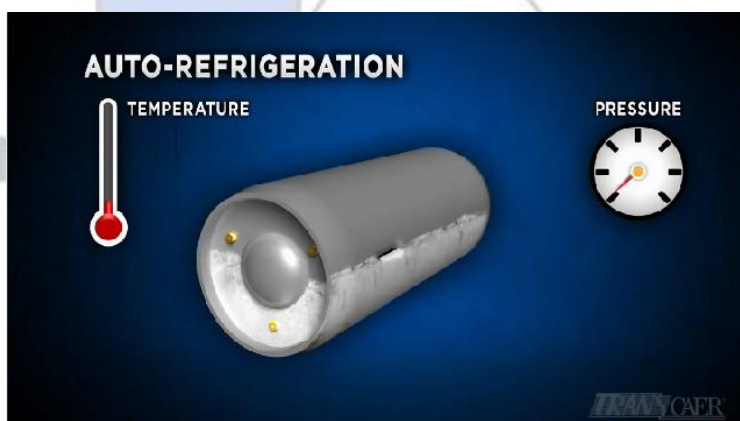
Fig. 5: Liquid chlorine has reached the boiling point and pressure drops to 0 psig
