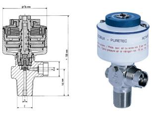
Since the valve seat is closed using springs, it can chatter open during transportation and handling. A manual lock forces the valve seat closed.
