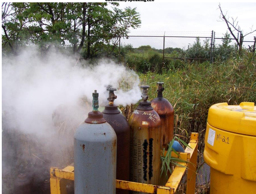
Fig. 1: HCl Cylinder Leak
