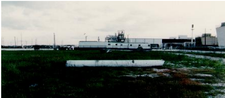
Fig. 11: Ruptured Tube Flew Over 800 ft
