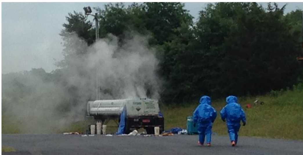
Fig. 13: Leaking Tube Trailer
