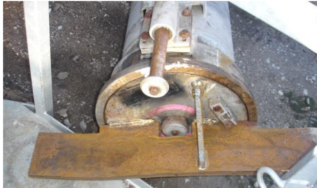
Fig. 5: Plate Welded Onto Door In Attempt to Open ERCV
