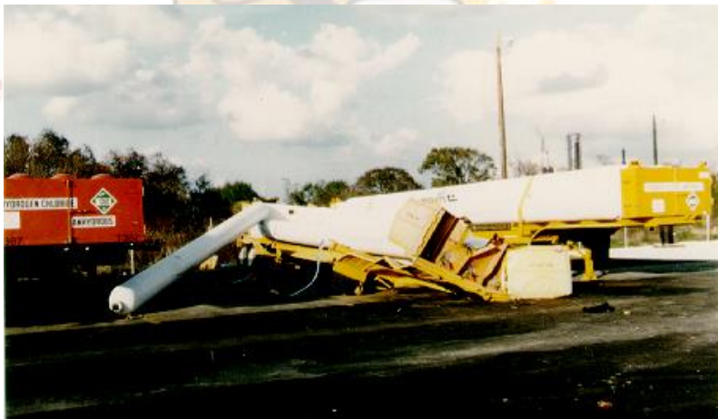
Fig. 11: Ruptured Tube Flew Over 800 ft
