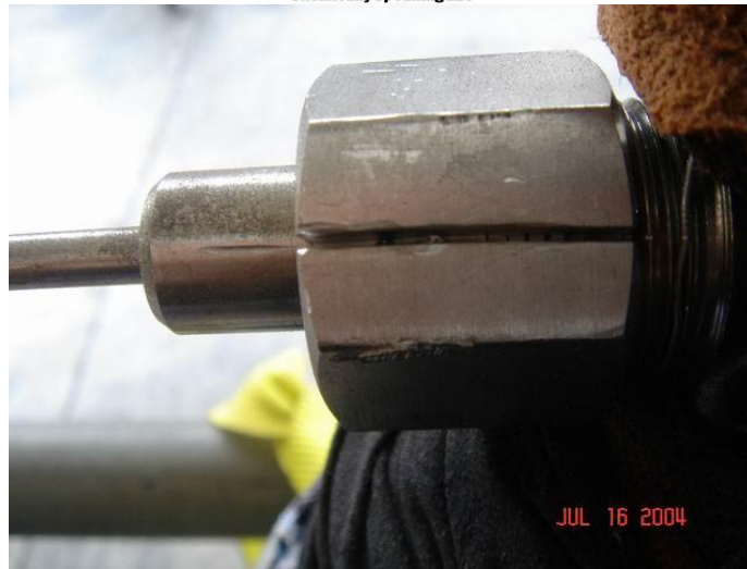
Photo of Nut cut on one side
