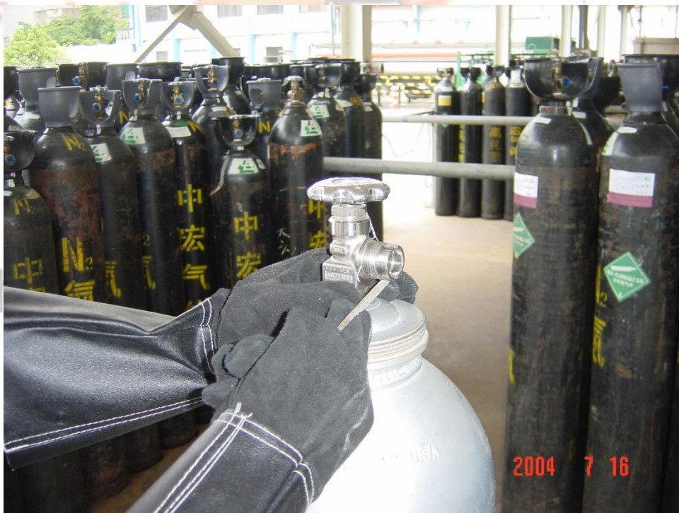
"Cleaning" or "dressing" the threads with jewelers file
