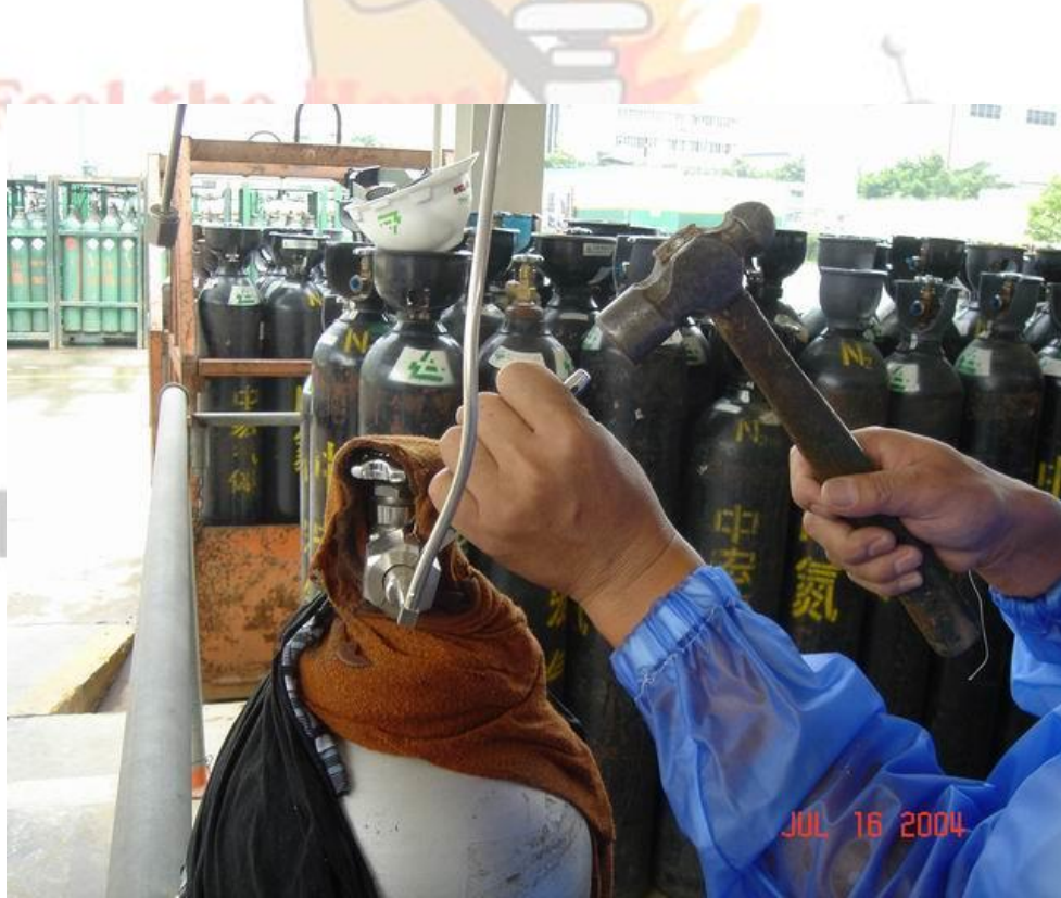
Splitting the nut with Chisel after cutting the nut with the grinder tool (but use gloves!).
