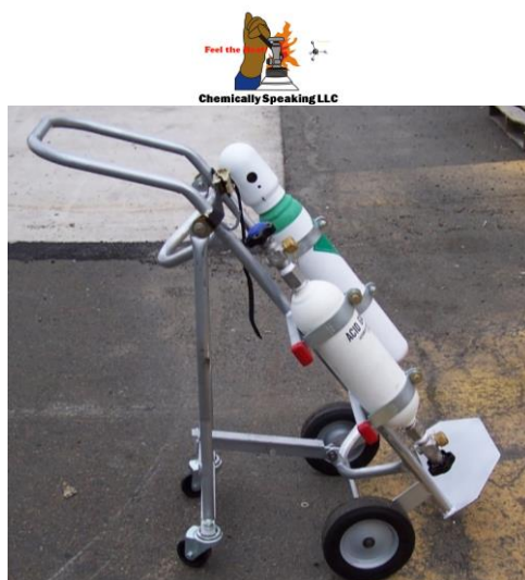
Fig.17: Leaking Cylinder Cap Cart (Photo by E. Ngai)
