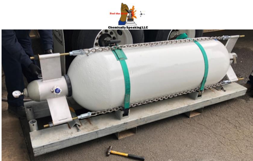
Fig. 6: Capping Kit Fully Assembled (Photos by E. Ngai)
