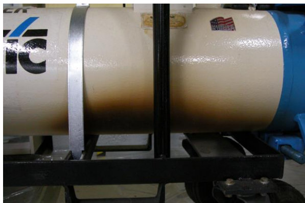
Fig. 26: \text{ClF}_3 Liquid Reaction With 5502 ERCV Bottom. (Photo by E. Ngai)
