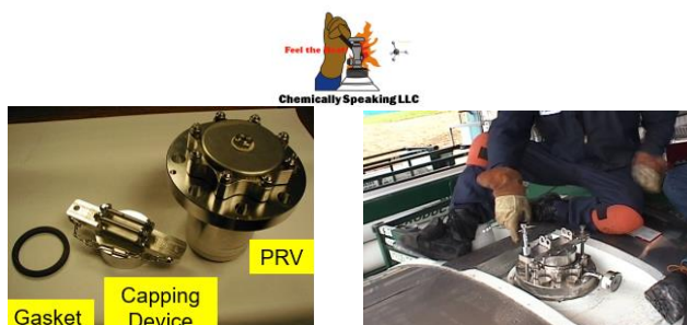
Figs. 9 & 10: Capping Device and PRV. Assembly of Capping Kit (Photos by E. Ngai)
