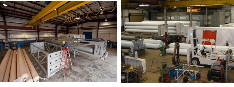
The tube skid built by FIBA is tshot blasted prior to painting and is to be painted with high quality industrial grade marine coating. Coating shall be performed in accordance with FIBA Procedure FIBA-P-23 for the skid frame and tubes. All required decals, placards, and markings to be installed by FIBA in accordance with DOT and international regulations. Customer supplied logos can be installed by FIBA in accordance with drawing and DOT and ISO regulations.
