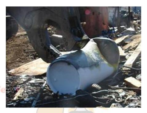
Chlorine ton cylinder that was not properly tested. The junk yard operator attempted to crush it. The release killed him.
