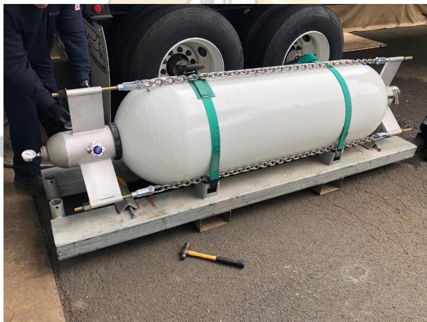
Y Capping kit for \text{NH}_3 , DCS, \text{Cl}_2
