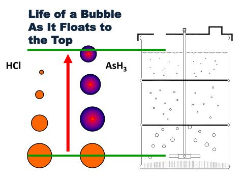
The HCl bubble will steadily decrease until it disappears while the AsH<sub>3</sub> bubble will only have surface reaction
