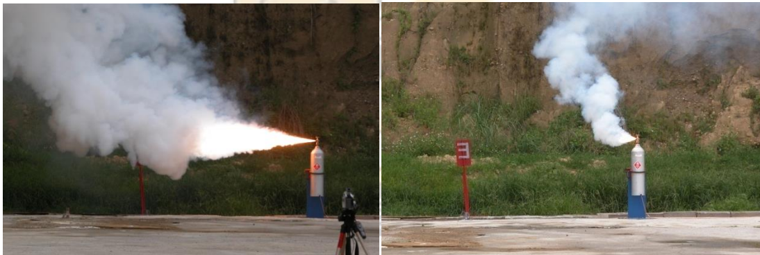
Silane Release without and with a 0.010" RFO, 1000 psig silane cylinder
