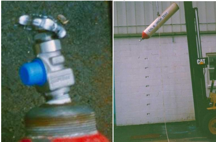
Valve Damage After Drop
