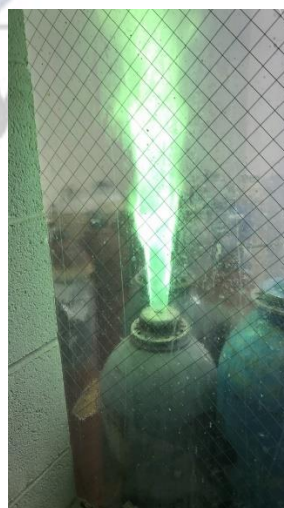
Fig. 6: Reaction of Boranes During Cleaning
