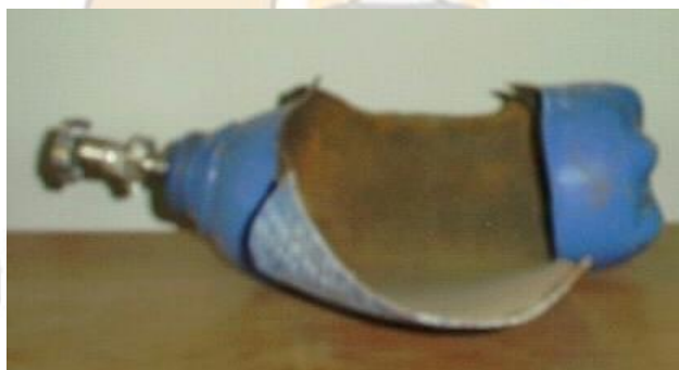
Fig 4: Cylinder Ruptured Minutes after Sodium Hydroxide Addition
