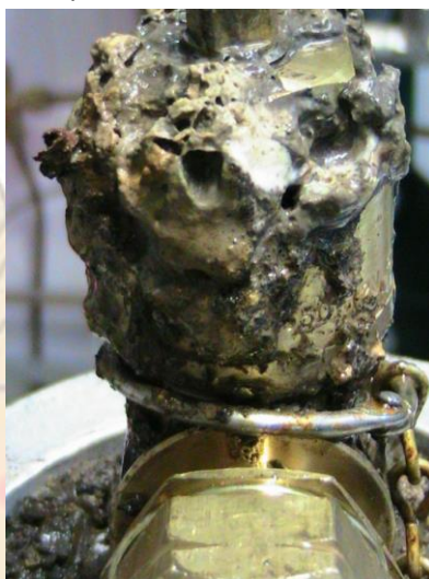
Fig 9: Melted Cylinder valve Handwheel
