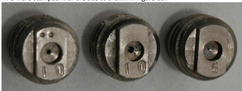
Fig.10: Superior Valve RFOs Stamped with Orifice Size
