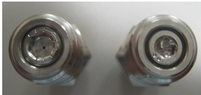
Figs 18: Rotarex, Notches and GasFlo, Dots
