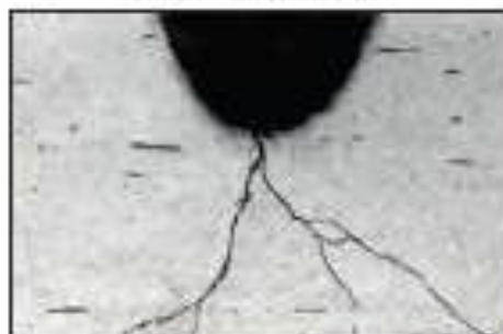
Figure 2: Transgranular cracks in a branching pattern (Source: (1) Maritich, R.)
