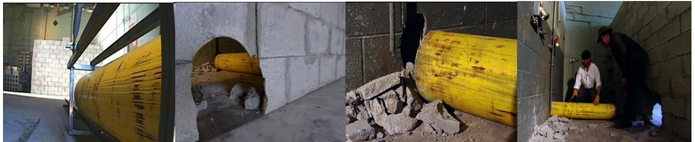
Fig 7 -10: Cylinder Impact of Concrete Block Wall
