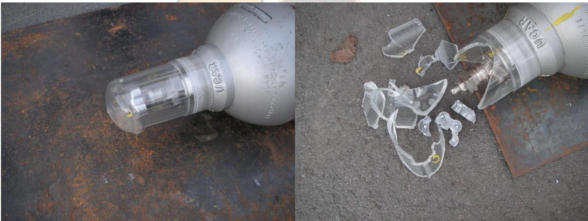
Figs 3 & 4: Polycarbonate Cylinder Cap Drop test
