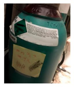
Figure 2. Illegally filled nitrogen cylinder.
