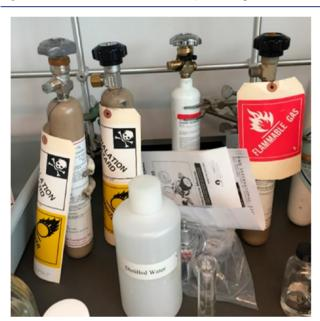
Figure 5. Lecture bottles containing highly toxic, oxidizer gases and flammable gas.
