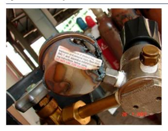
Figure 10. Regulator used for another gas service was adapted for oxygen use; it exploded when the cylinder valve was opened.
