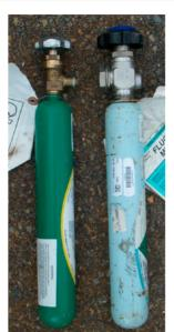
Figure 4. Lecture bottle (left) and 7X cylinder (right).
