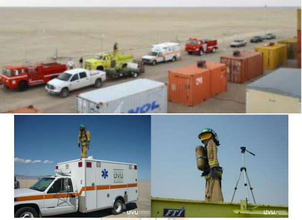
The vehicles even after 5 exposures to high Cl<sub>2</sub> levels still ran. The turnout and SCBA were deonned and appeared to be unaffected. Concluded that a emergency responder would be protected and be able to escape a worse case Cl<sub>2</sub> release.
