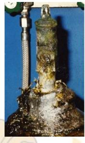
A full 150 lb cylinder contains 150 lbs of liquefied Chlorine Gas The gas specific volume of  $Cl_2$  at 70°F is 5.39 ft<sup>3</sup>/lb 5.39 ft<sup>3</sup>/lb x 150 lbs = 808.5 ft<sup>3</sup> of gas 808.5 ft<sup>3</sup> x 28,315 cc/<sup>ft3</sup> = 22,892,677 cc At a leak rate of 50 cc/min this will leak for 457,854 minutes (318 days)!
