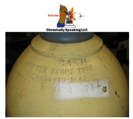
High pressure seamless cylinders (3AA) are designed to withstand bullet penetration without catastrophic failure even when pressurized to the working pressure
