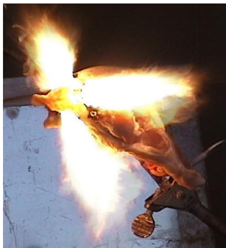
Fig. 3: \text{ClF}_3 Vapor and Raw Chicken
