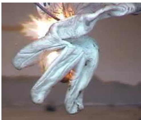
Fig 1: \text{ClF}_3 Gas and New Leather Gloves
