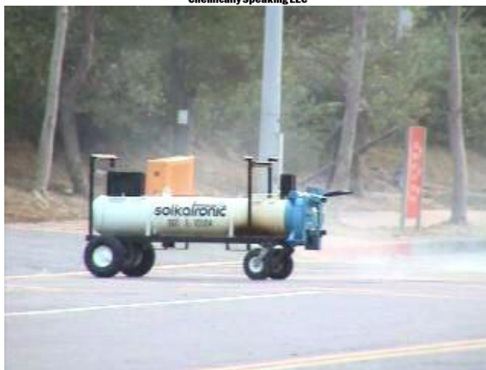
ERCV With \text{ClF}_3 Liquid Reacting With Carbon Steel
