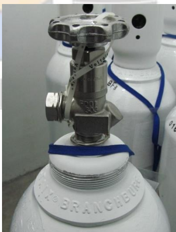
Fig. 2: Cylinder Valve Wire Tied
